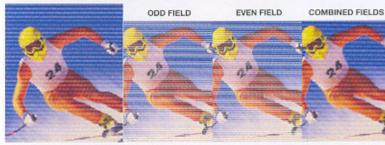
Traditional interlaced video sends the odd/ even fields separately for higher resolution with lower bandwidth
